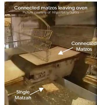
formed and baked. After the dough is kneaded, it is rolled into a long, flat sheet which passes under two sets of blades that score the sheet lengthwise and widthwise. These blades score the sheet into *matzah*-sized squares but do not cut the dough all the way through; rather, the *matzah* passes through the oven as a scored sheet, and after it leaves
